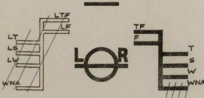
to certify that this ship has been surveyed and the freeboards and load lines shown above have been assigned in accordance with the Convention.
