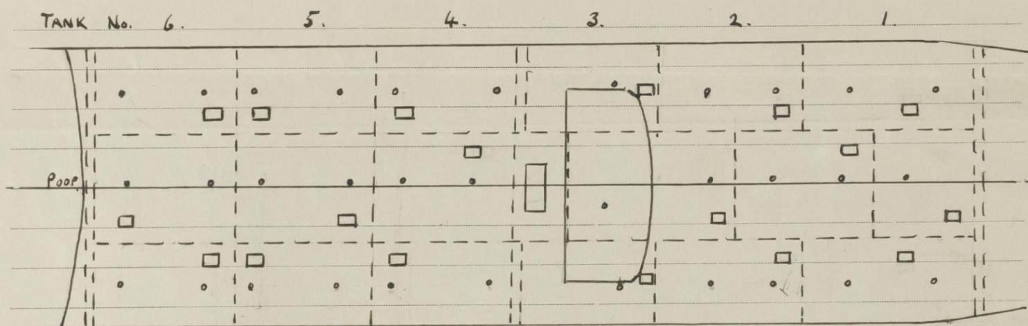
Deck doubling fitted at Butterworth openings which are abreast cargo hatches.
