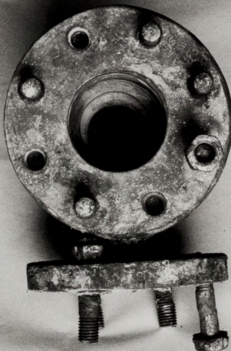
STOP CHECK VALVE BODY STBD. BOILER
