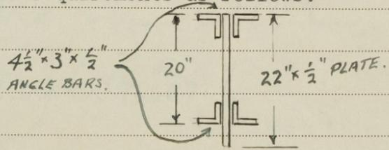
Nos. 2 and 3 hatchways on the bridge deck and freeboard deck and No. 4 hatchway on the raised quarter deck have 3 fore and afters each spaced 5'-1-1/2" as per sketch
