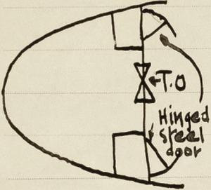
The arrangement of the poop bulkhead (in the tonnage well) is as shewn on the accompanying sketch. Two hinged steel doors (4'6" x 2'6") are fitted to the wing stores as shewn on the accompanying sketch in addition to the tonnage opening on the centre line.
