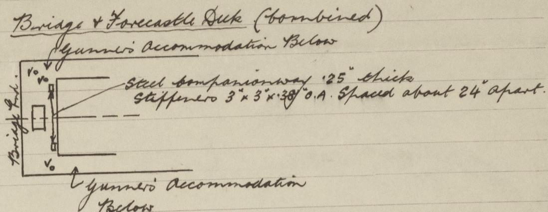
Entrance to gunner's accommodation port & starboard. Solid wood door with 18" coaming above bridge decks. (Fitted in Steel Companionway)
