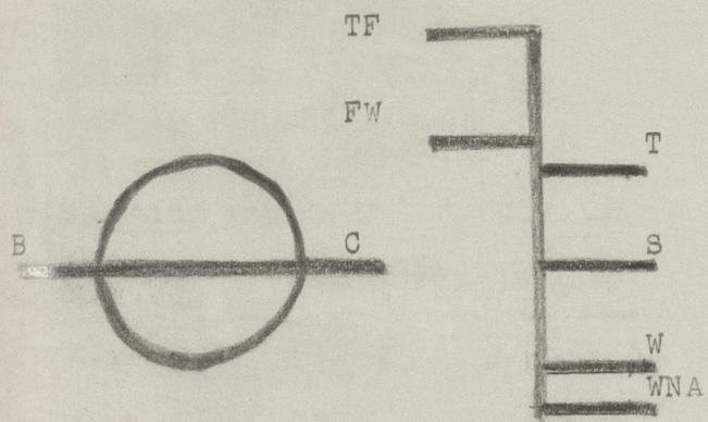
...er edge of the deck line from which these freeboards are measured is          inches above the top of the stringer plate on the deck at side.
