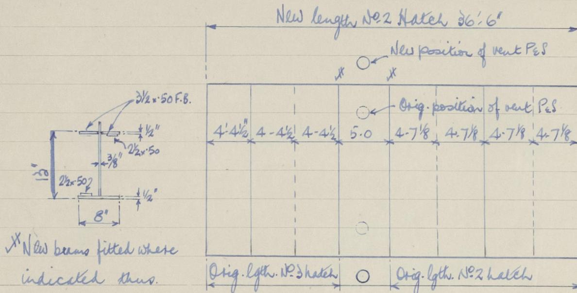
The 18" dia. No.2 Hold ventilator originally fitted in the well between No.2 & No.3 upper deck hatches (p&s), now removed & refitted abreast No.2 hatchway opening p&s. Vent coaming 36" above wood deck sheathing x 3/8" thick supplied with wood plug & canvas cover and upper deck opening suitably reinforced in way
