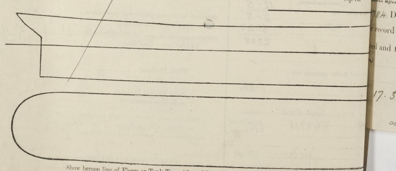
Show hereon line of Floors or Tank Top with position of any Breaks in same; also height of Peak Tank top
