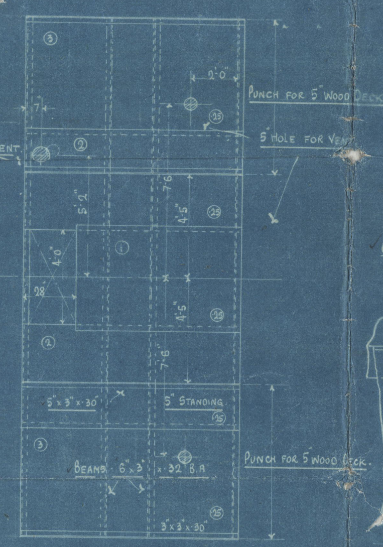
DETAIL OF BRIDGE DECK
