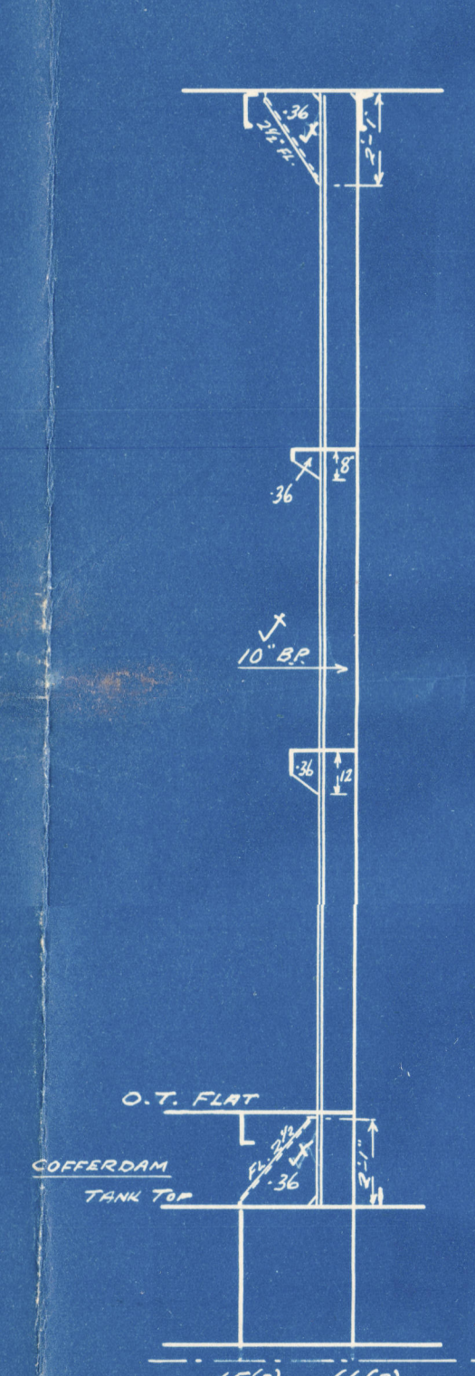
BULKHEAD STIFFENERS ON FRs. 66 (P) 67 (S)
