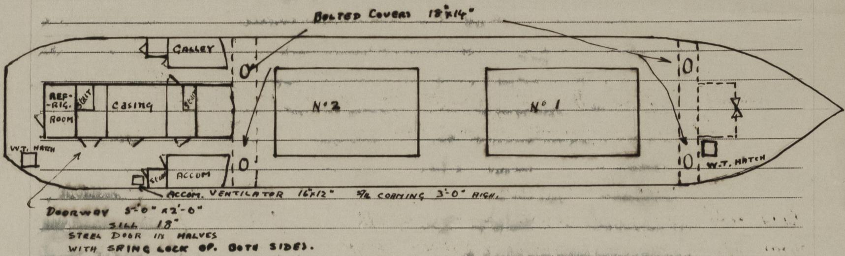
copper bands fitted at each end of tween deck and after end of hold to water seal hold when carrying petroleum in steel containers.
