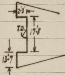
BRIDGE After coal hatch on bridge deck P. & S. reduced in size at aft end. Length of hatch now 14'-7" Deck in way of removed portion of hatch efficiently plated over.
