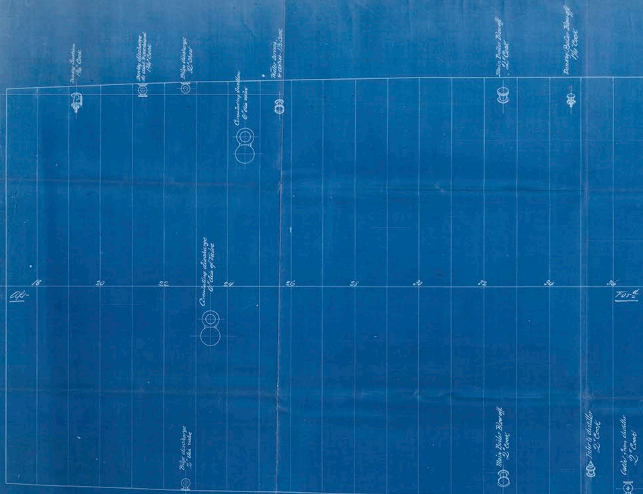
Position of Cocks & Valves on Ships Side — in Engine & Boiler Rooms — Scale: 1/2" to a foot
