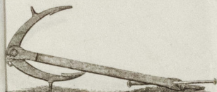
FIG. 1-Position of the Anchor when canted.
