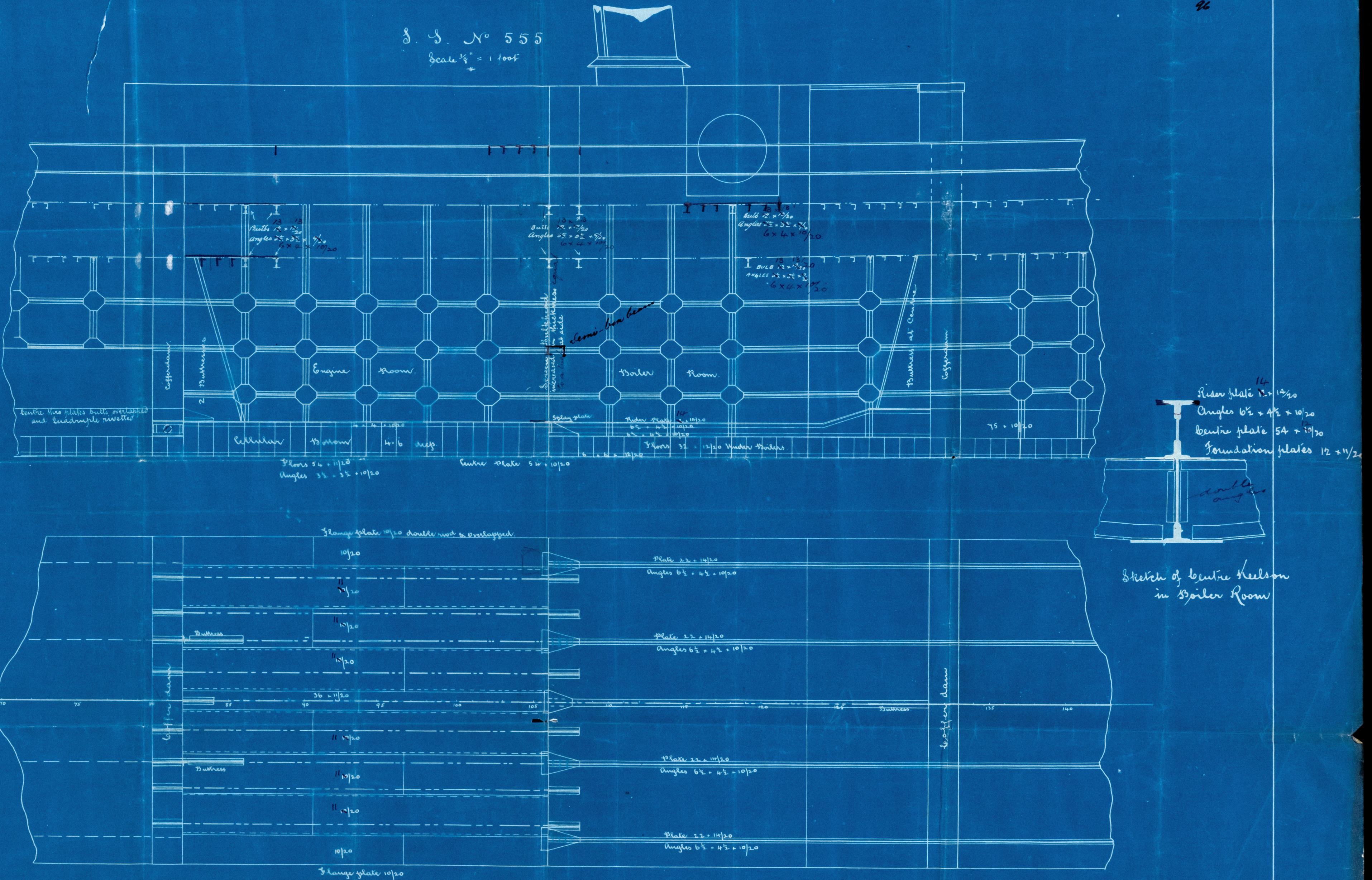
Bottom of bulk top overlapped and double riveted.
