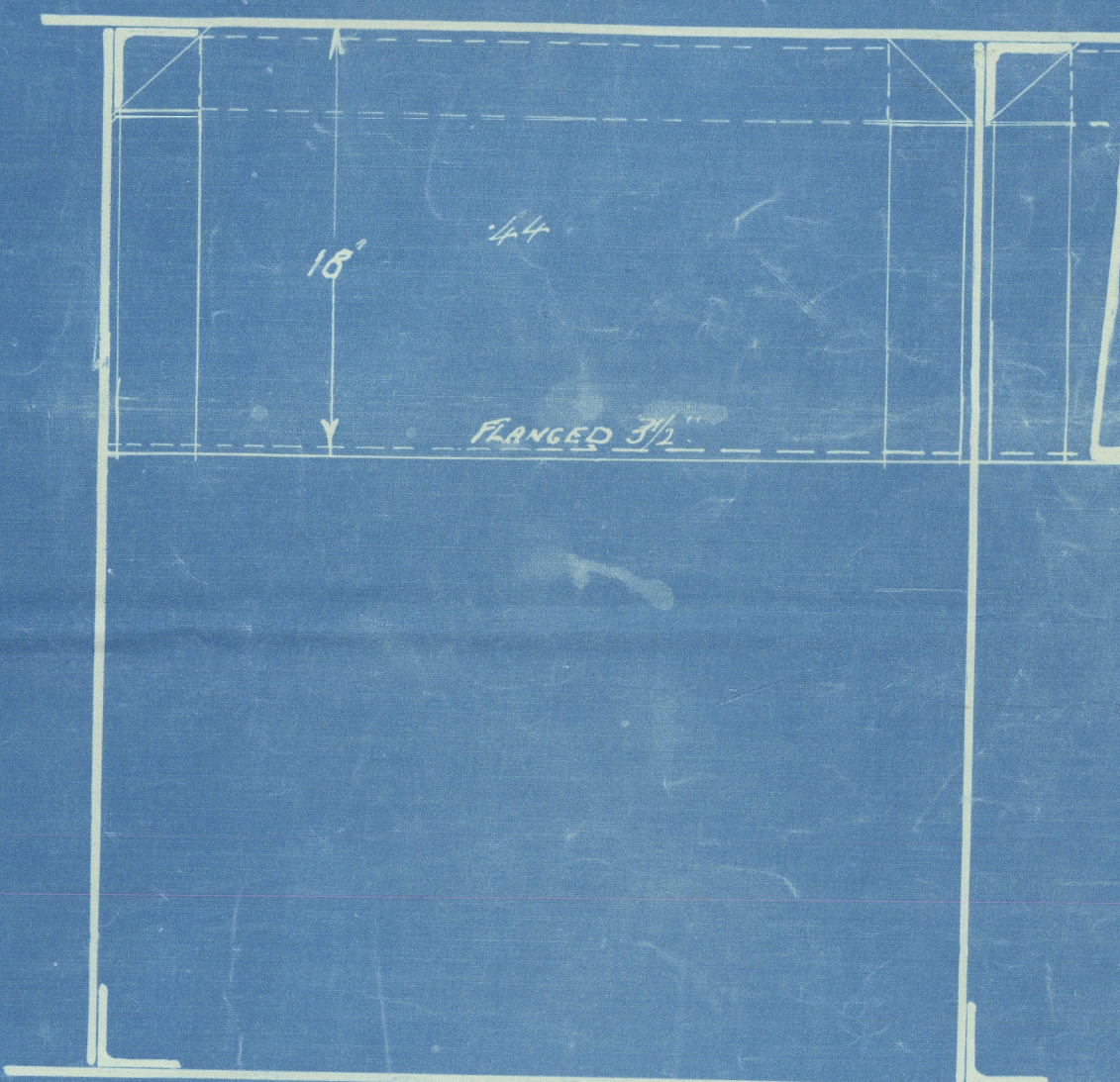
TYPICAL SECTION OF NEW HALF INTERCOSTALS
