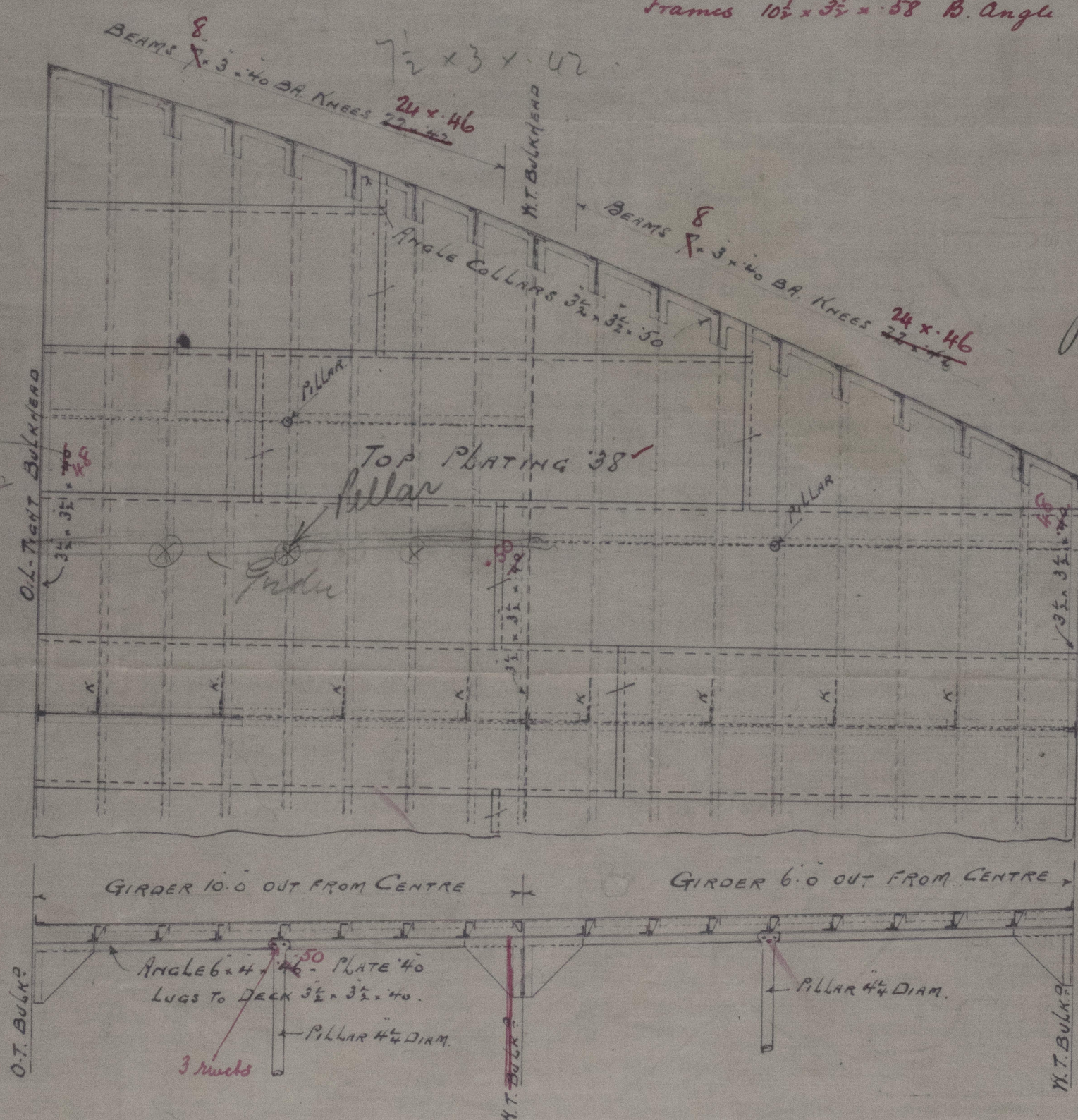
No 165 BULKHEAD (LOOKING FORWARD.)
